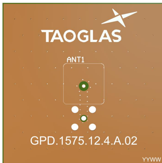
Top Side (GP.1575.12.4.A.02 placement on 50x50mm PCB)
