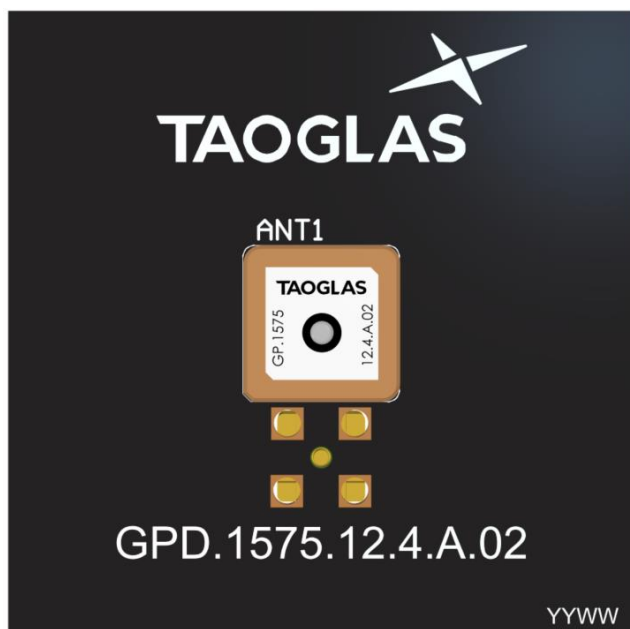
Top Side (GP.1575.12.4.A.02 placement on 50x50mm PCB)
