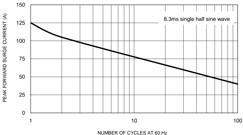
Fig.5 Maximum Non-Repetitive Forward Surge Current
