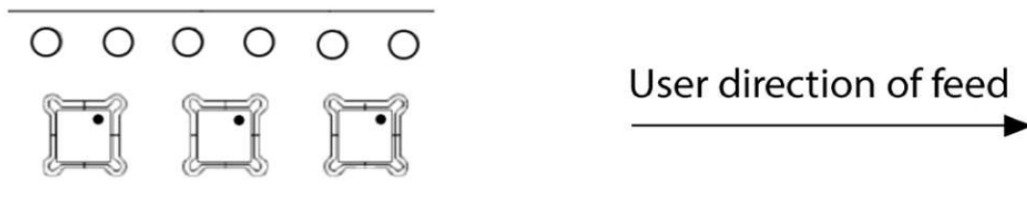
Figure 29. Package orientation in carrier tape
