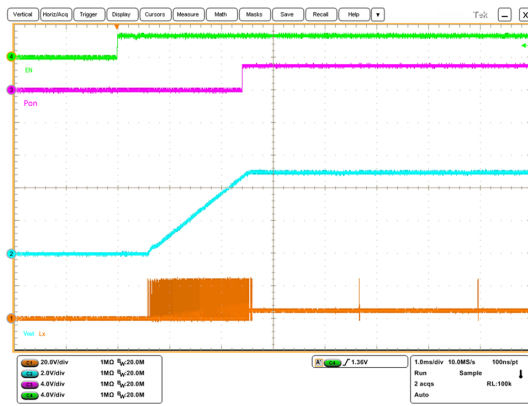
Figure 28. Enable startup (Vin = VCC = 24 V, Vout = 0x64 (5 V), no load)
