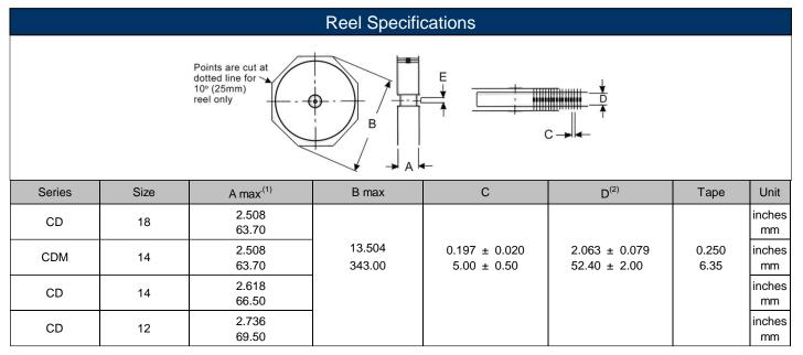
Dimension "E": This is a non-critical dimension that does not have a tolerance in the standard.
