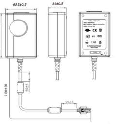
12V Models Output Connector: 6 Pin Molex 39-01-2060 or equiv. Pins 1,4 = (+), Pins 3,6 = (-), Pins 2,5 = NC
