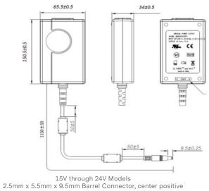
3. The unit should not be covered or enclosed to protect against excessive case temperature rise.
