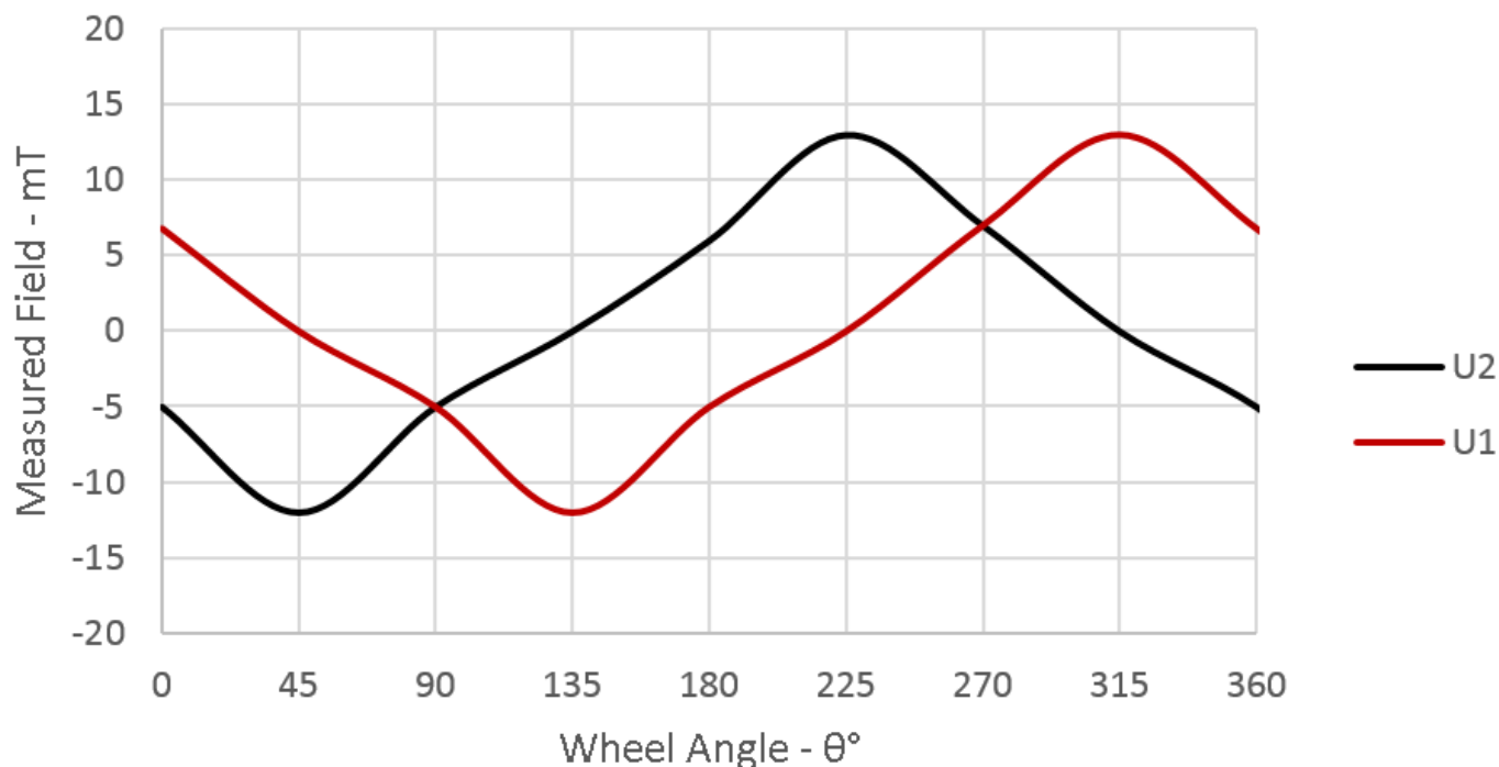
Figure 1.4. Magnetic Field Strength vs. Angle Position
