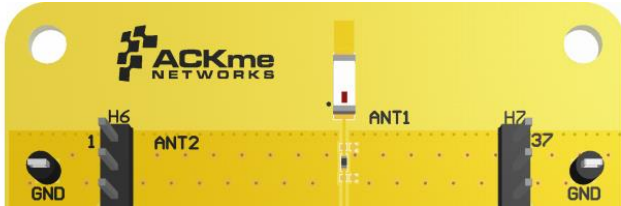
Figure 11 – Chip antenna layout example
