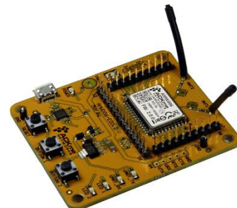
Figure 10 - AMW006-E03 eval board with wire antennas
