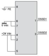
With External Device Monitoring (EDM) feedback loop
