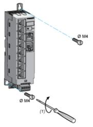
(1) Maximum tightening torque: 1,7 Nm / 15 lb-in.
