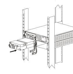
Slide the left hand side battery module into the XLBP.
