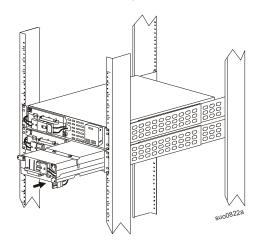
Connect the two XLBP connectors from the enclosure to the two RBCs. See "XLBP Connectors Installation" on page 8.
