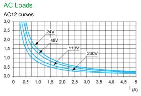
AC12control of resistive loads and of solid state loads isolated by optocoupler,  $\cos \phi \ge 0.9$ .
