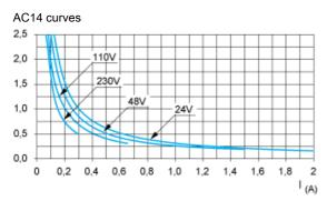
AC14control of small electromagnetic loads  $\leq$  72 VA, make: cos  $\phi$  = 0.3, break: cos  $\phi$  = 0.3.
