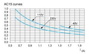
AC15control of electromagnetic loads > 72 VA, make:  $\cos \phi = 0.7$ , break:  $\cos \phi = 0.4$ .
