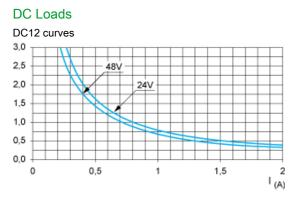
DC12control of resistive loads and of solid state loads isolated by optocoupler,  $I/R \le 1$  ms.
