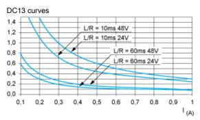
DC13switching electromagnets, L/R ≤ 2 x (Ue x Ie) in ms, Ue: rated operational voltage, Ie: rated operational current (with a protective diode on the load, DC12 curves must be used with a coefficient of 0.9 applied to the number in millions of operating cycles)
