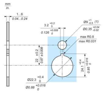
(1) : For IP X9 applications, the max recommendation dimension of hole is  $\emptyset 9$  mm/ $\emptyset 0.35$  in.
