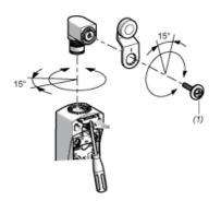
(1) Tightening torque (Min: 1) (Max: 1.5)
