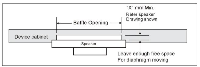
movement. The minimum distance required, "X," is the dimensioned drawing below is 3.0mm.
