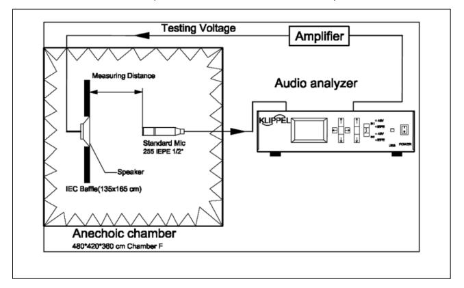
**Measurement Method** (measured with  $P_{DRIVE} = 1.0W$ , distance = 0.5m)
