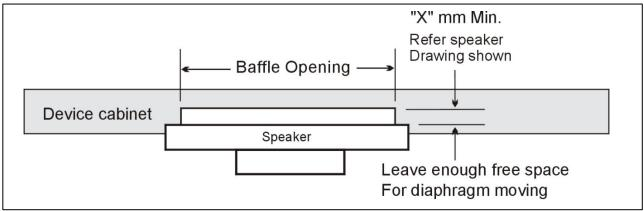
movement. The minimum distance required, "X," is the dimensioned drawing below is 2.0mm.
