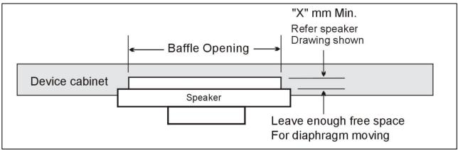
movement. The minimum distance required, "X," is the dimensioned drawing below is 0.5mm.
