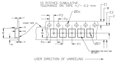
REEL DIMENSIONS А inches 7.0 10.0 13.0 mm 177.8 254.0 330.2 в 2.50 inches 4.00 3.75 63.5 101.6 95.3 Tape Width mm С 13.0 +0.5 / -0.2 mm 16.4 +2.0 -0.0 D mm 16.4 16.4 16.0 +2.0 -0.0 +2.0 -0.0
