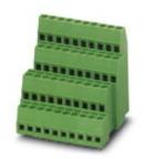
PCB terminal block, nominal current: 15 A, nom. voltage: 400 V, pitch: 5.08 mm, number of positions: 14, connection method: Screw connection, mounting: Soldering, conductor/PCB connection direction: 0 °, color: Pebble gray
