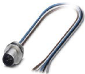
Sensor/actuator flush-type plug, 5-pos., M12, A-coded, front/screw mounting with Pg9 thread, with 1.0 m TPE litz wire, 5 x 0.34 mm 2
