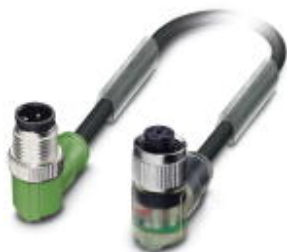
Sensor/actuator cable, 3-position, PUR halogen-free, black-gray RAL 7021, Plug angled M12, A-coded, on Socket angled M12, A-coded, with 2 LEDs, cable length: 2.5 m
