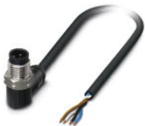
Sensor/actuator cable, 4-position, Special mixture on PVC base, black RAL 9005, Plug angled M12, A-coded, on free cable end, cable length: 10 m
