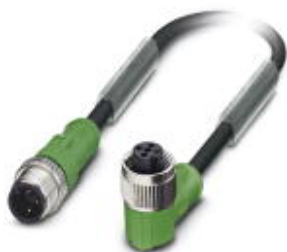
Sensor/actuator cable, 3-position, PUR halogen-free, black-gray RAL 7021, Plug straight M12, A-coded, on Socket angled M12, A-coded, cable length: 0.6 m
