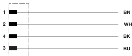
Contact assignment of M12 plugs / sockets bridged
