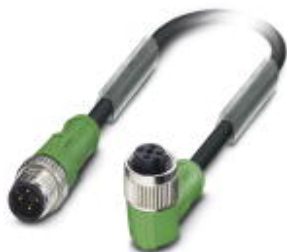
Sensor/actuator cable, 4-position, PUR halogen-free, black-gray RAL 7021, Plug straight M12, A-coded, on Socket angled M12, A-coded, cable length: 7 m
