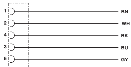
Contact assignment of the M12 socket
