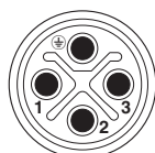
M12 plug pin assignment, 4-pos., S-coded, plug side view
