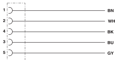
Contact assignment of the M12 socket
