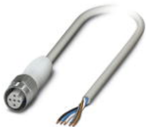
Sensor/actuator cable, 5-position, PP-EPDM halogen-free, gray RAL 7035, cable length: 20 m, Hygienic design, with high-grade steel knurl
