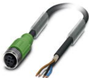
Sensor/actuator cable, 4-position, PUR halogen-free, black-gray RAL 7021, shielded, free cable end, on Socket straight M12, A-coded, cable length: 15 m, Shield not connected to knurl
