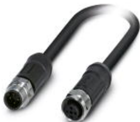
Sensor/actuator cable, 4-position, PE-X/PE-X, black-gray RAL 7021, Plug straight M12, A-coded, on Socket straight M12, A-coded, cable length: 100 m, for outdoor applications, with high-grade steel knurl
