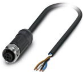
Sensor/actuator cable, 4-position, PE-X halogen-free, black-gray RAL 7021, free cable end, on Socket straight M12, A-coded, cable length: 20 m, for outdoor applications, with high-grade steel knurl
