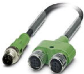
Sensor/actuator cable, 4-position halogen-free, yellow, Plug angled M12 SPEEDCON, A-coded, on Socket straight M12 SPEEDCON, A-coded and Socket straight M12 SPEEDCON, A-coded, cable length: 1.5 m
