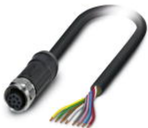
Sensor/actuator cable, 8-position, PE-X halogen-free, black-gray RAL 7021, free cable end, on Socket straight M12, A-coded, cable length: 1 m, for outdoor applications, with high-grade steel knurl
