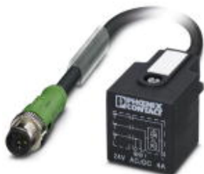
Sensor/actuator cable, 3-position, PUR/PVC, black RAL 9005, Plug straight M12, A-coded, on Valve connector A, with 1 LED, connected with Z diode, cable length: 6 m
