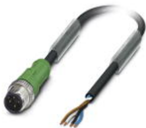
Sensor/actuator cable, 4-position, PUR halogen-free, gray RAL 7001, Plug straight M12, A-coded, on free cable end, cable length: 1 m
