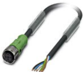
Sensor/actuator cable, 5-position, PUR halogen-free, black-gray RAL 7021, free cable end, on Socket straight M12 SPEEDCON, B-coded, cable length: 2 m
