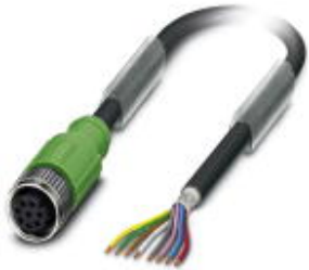
Sensor/actuator cable, 8-pos., PUR, halogen free, RAL 7021 (black gray), shielded, free cable end, to straight M12 socket, A-coded, cable length: 100 m, high-grade steel knurl
