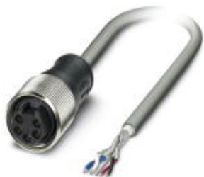
Bus system cable, DeviceNet, 5-pos., PUR, halogen-free, RAL 7001 (gray), straight M12 male plug, to straight 7/8" 16UNF female plug, cable length: 1 m
