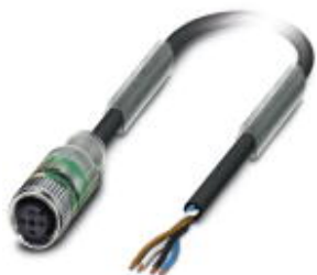
Sensor/actuator cable, 4-position, PVC, gray RAL 7001, free cable end, on Socket straight M12, A-coded, with 2 LEDs, cable length: 10 m
