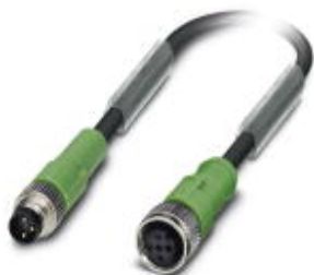
Sensor/actuator cable, 3-position, PUR halogen-free, black-gray RAL 7021, Plug straight M8, on Socket straight M12, A-coded, cable length: 3 m
