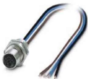
Flush-type connector, Power, 4-position, Socket, M12, L - Power, Rear mounting, M16 x 1.5, Individual wires, cable length: 1.5 m, 2.50 mm 2 , PEX litz wire
