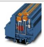
Knife disconnect terminal block, With test socket screws for insertion of test plugs, nom. voltage: 400 V, nominal current: 8 A, connection method: Screw connection, cross section: 0.2 mm² - 4 mm², AWG: 24 - 12, length: 76.5 mm, width: 6.2 mm, color: blue, mounting: NS 35/7,5, NS 35/15, NS 32
