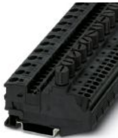
Fuse terminal block for cartridge fuse insert, cross section: 0.5-10 mm 2 , AWG: 20-8, width: 12.2 mm, color: Black
