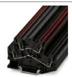
Component terminal block, with integrated diode, nom. voltage: 500 V, nominal current: 22 A, connection method: Spring-cage connection, cross section: 0.08 mm² - 4 mm², AWG: 28 - 12, length: 78 mm, width: 5.2 mm, color: black, mounting: NS 35/7,5, NS 35/15
