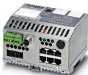
Ethernet Smart Managed Compact Switch with six 10/100 Mbps RJ45 ports and two 1000 Mbps SFP slots
