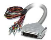
Assembled shielded round cable; connection 1: Single wires (25-position) (The wires are marked and fitted with ferrules); connection 2: D-SUB pin strip (1x 25-position); cable length: 5 m
