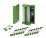
Termination carrier for redundantly connecting 16 MACX Analog Ex i signal conditioners to analog output cards of the Yokogawa Centum VP controller, via two KS40 connectors, 40-pos. Suitable for Yokogawa card AAI543.
