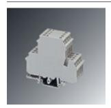
Feed-through terminal block, With test socket screws for insertion of test plugs, nom. voltage: 400 V, nominal current: 26 A, connection method: Screw connection, cross section: 0.2 mm² - 4 mm², AWG: 24 - 12, length: 80 mm, width: 6.1 mm, color: gray, mounting: NS 35/7,5, NS 35/15, NS 32
